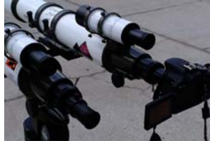
Figure 14: A close up view of the mounting of the camera directly in the telescope in place of the eyepieces [16].
